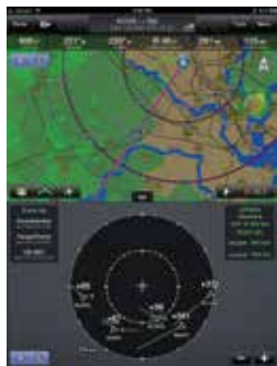
With an optional GDL 39 or 39 3D ADS-B receiver, Garmin Pilot can display subscription-free weather and datalink traffic. Traffic displays with our patent-pending TargetTrend™ technology that shows traffic trajectories relative to your aircraft.
