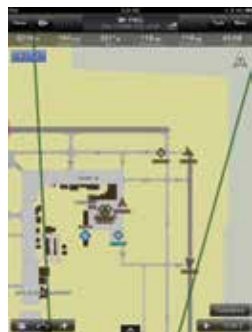
Optional SafeTaxi® diagrams with geo-referencing capability help you navigate on unfamiliar airports. With an optional GDL 39 receiver, TerminalTraffic™ technology displays ADS-B equipped surface targets right on these diagrams.
