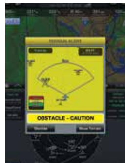
A terrain and obstacle database provides high-resolution contour mapping to show your aircraft's proximity to potentially hazardous terrain or obstacles like towers, as well as provide audible and visual cautions and warnings as you near these obstructions.
