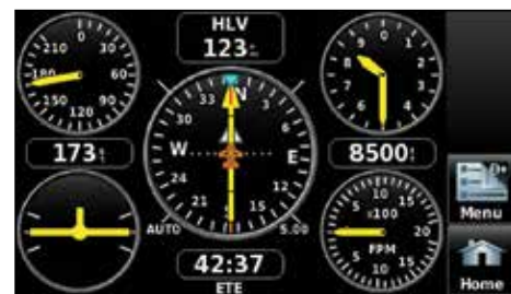
Fast 5 Hz update rate provides smoother, more responsive readouts on GPS-derived "Panel" page
