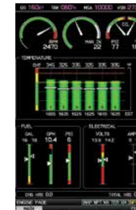
Detailed Engine Indication System (EIS) readouts can be viewed by selecting the ENG page
