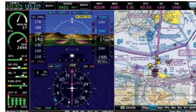
Detailed VFR Sectional charts, as well as Low- and High-Altitude IFR Enroute charts, can be displayed in the navigation window of your G3X Touch display
