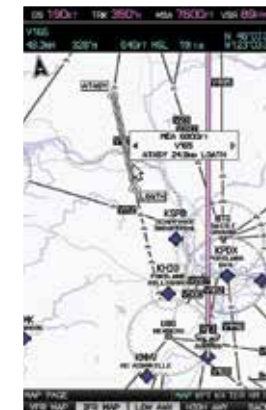
IFR map mode displays Victor airways and Jet routes, derived from navigation database
