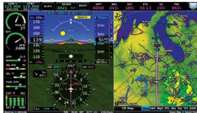
Optional Sirius XM™ satellite weather can overlay on the G3X Touch moving map 2
