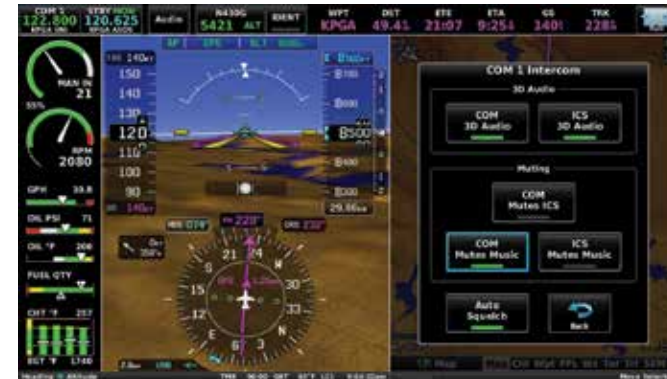
G3X™ Touch offers on-screen control for remote comm, transponder and two-place intercom functions with 3D audio, stereo music input and more
