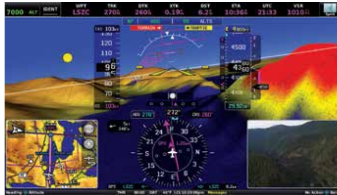
Inset frames on the G3X™ Touch flight display let you view a continuous video feed from optional VIRB® action cameras – along with moving map detail, SVX synthetic vision and ADS-B traffic targets
