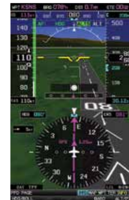
SVX shows runway surfaces, numbers and thresholds in virtual 3-D
