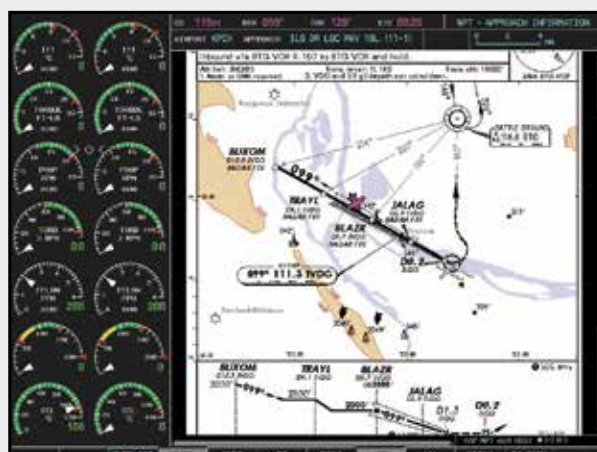
Optional ChartView™, powered by Jeppesen, lets pilots accurately overlay their aircraft's position on approach procedures and airport diagrams. Standard Instrument Departure and Arrival charts (SIDs and STARs) are also provided.
