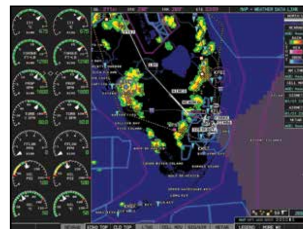
Weather datalink capability, via SiriusXM™ Satellite Weather service, provides the G1000 with color NEXRAD, METARs, TAFs, lightning, and other U.S. data displays (subscription required).
