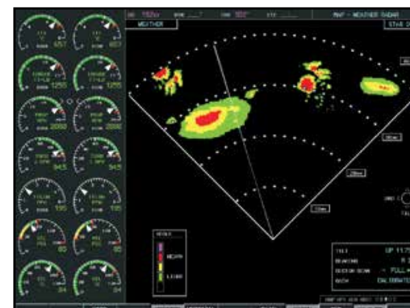
For onboard weather analysis, the King Air package features Garmin's all-digital, fully stabilized GWX™ 70 color radar. It provides reduced power consumption and extended life in comparison to previous generations of magnetron-based radars.
